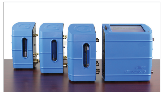
High, standard, & low flow cell modules are easily interchanged
