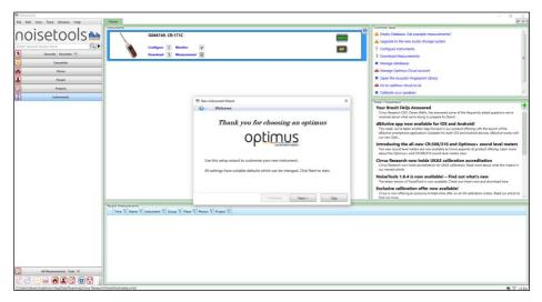
When you connect an Optimus sound level meter for the first time, you'll be prompted to use the New Instrument Wizard to customise its settings. This will allow you to set the language, date and time, and brightness settings, as well as configuring the meter for repeat measurements (if required/available).
